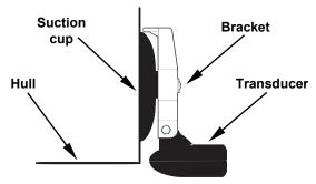
Portable transducer installed on boat transom.
